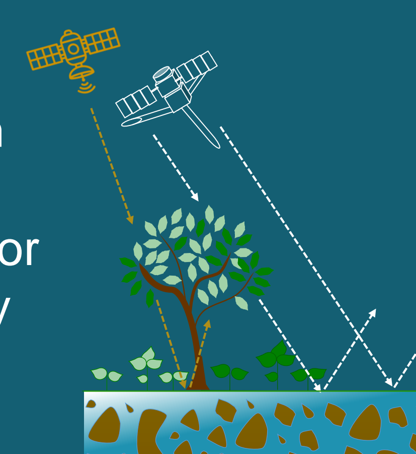
Figure 3: Vegetation water content is an error source for soil moisture retrieval. Furthermore, the harmonization of different sensors techniques is important for data comparability.
