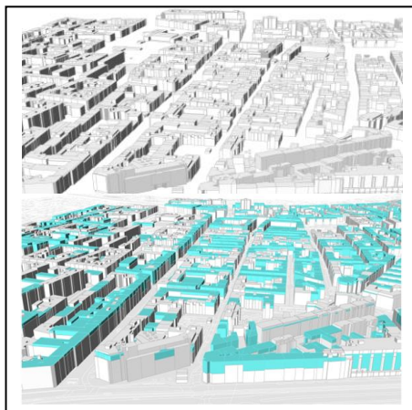
Figure 1: Building structure and densification potential in Vienna's 12 th district. Top: current building structure; bottom densification scenario according to the Vienna zoning plan. (Sources: AIT: 3D model, densification scenario, Wien MA18; height zoning map)
