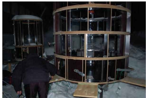
Fig. 2 – Dendrite generator snow is produced in a container
