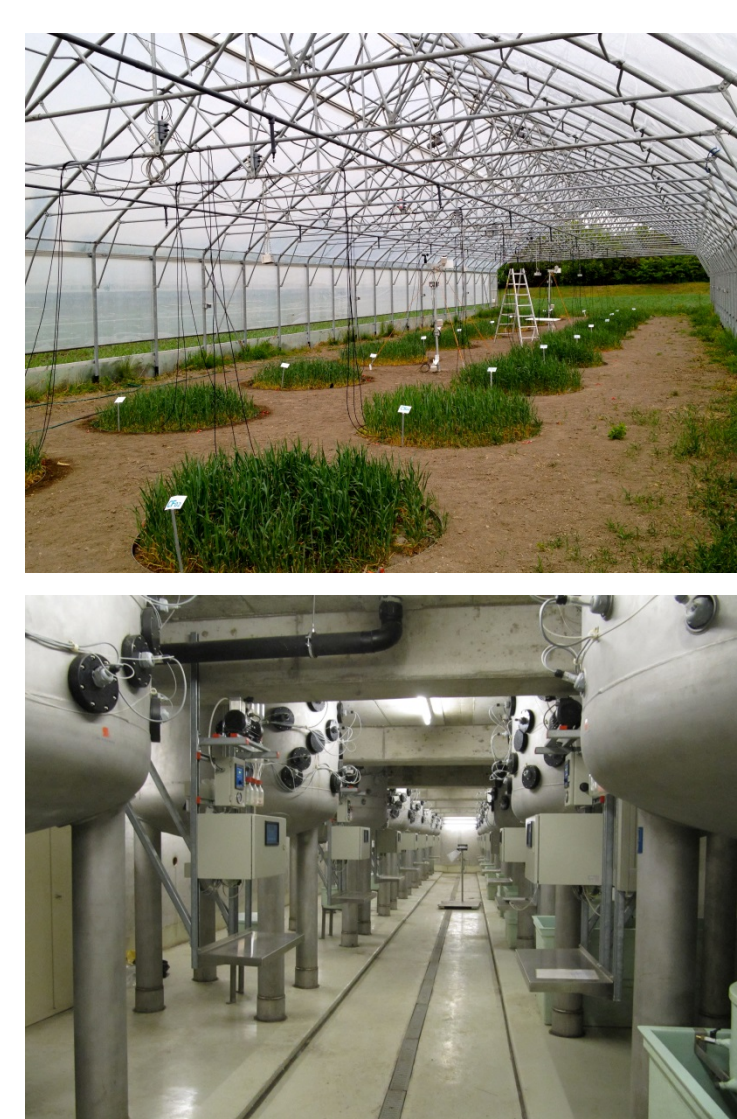
Fig. 1. Lysimeter site at AGES Vienna: Experimental plots (above) and basement of lysimeters (below)
