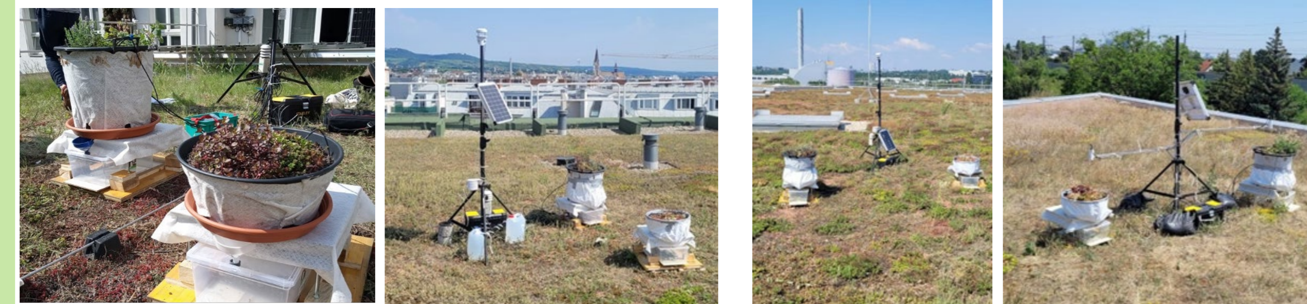
Fig. 1: Final setup of the experimental units covered up with white foil at the non-irrigated setups at the sites (a) KAN, (b) AKH, (c) REW, (d) JAE.
